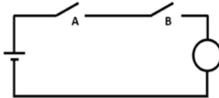
Q1. (i) Switch A and switch B are said to be *in series*. Based on your knowledge of a closed circuit, when do you think the bulb will light up?
